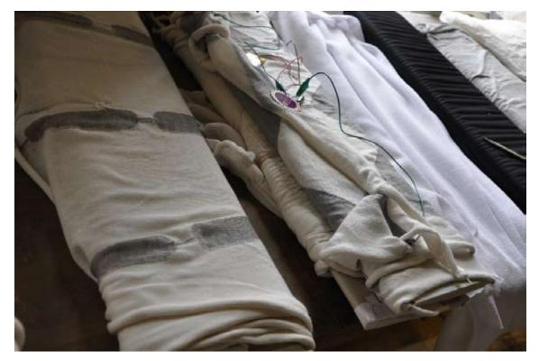
figure 1. Smart-textiles capable of measuring stretch developed in STS project, hooked up to a LilyPad Arduino
